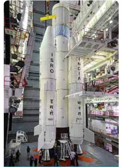
Two L40 strap-ons attached to the GSLV-F05 first stage core during launch vehicle integration
